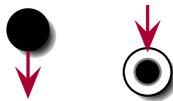
Figure 69: Example of activity diagrams start and end nodes
